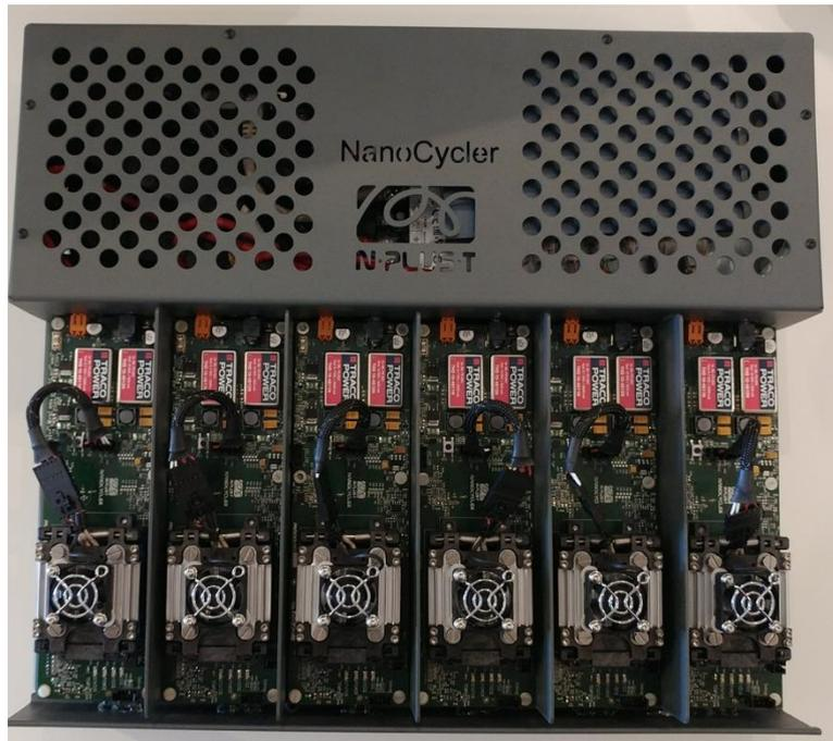
*Figure 4 NplusT's NanoCycler NAND characterization equipment*
