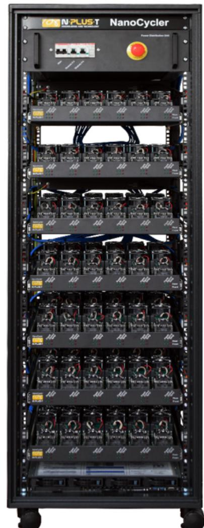
Since each Tester Unit directly connects with a single NAND device, and a NAND device contains up to 16 dies (HDP package), the NanoCycler full system configuration can test up to 1344 NAND dies concurrently.
